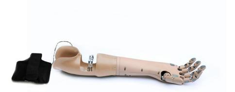
Developed with funding from Wellcome Trust (UK), PURAK-prosthesis provides *functionality with affordability*. With its *single* motor driven fully articulated structure controlled by a novel *myo-mechanical* control interface, it can adaptively grasp arbitrary shapes and let the user *feel the grasp force* too! It weighs just 500gm and costs less than a 10<sup>th</sup> of its competition.
