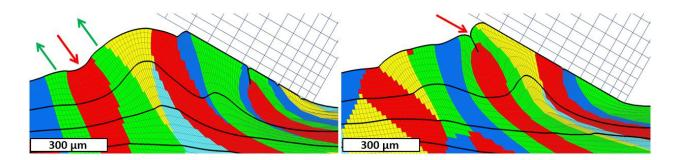
Microstructural effects can produce unexpected surface damage during deformation processing of metals via surface fold formation. Two frames from a finite element (FE) simulation depicting a surface depression (a), which then forms a surface fold (b), in sliding of aluminum-1100 modeled as a heterogeneous polycrystalline aggregate. The fold eventually becomes a crack-like damage feature on the residual surface.
