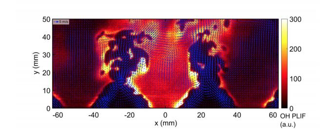
The image captures the instantaneous velocity and reactive species fields inside a model gas turbine combustor. This is experimentally obtained by simultaneous Particle Image Velocimetry and Planar Laser Induced Fluorescence of hydroxyl (OH) radical. In the image, the blue arrows represent flow velocity vectors corresponding to the turbulent swirling flow and the color scale represents the OH fluorescence intensity, respectively.
