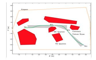
The figure above showcases results from a novel continuous curvature path planning methodology for Unmanned Aerial Vehicles (UAVs) developed using four parameter logistic curves. Fig A presents the scenario with an airspace defined in the IISc north area and restrictions within the airspace modeled as convex polygons. Fig B presents the planned (dashed curve) and followed path (solid line) connecting four waypoints using a simulation.
