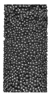
Naturally occurring geomaterials such as sandstones, soft rocks, are comprised of particulates, often held together by cohesion between them. The geology, surrounding environs bring forth this cohesion between the particulates. We study the structure and mechanical behaviour of such cohered granular materials at multiple length scales. The figure presents an x-ray computed tomography image of a cemented granular ensemble.
