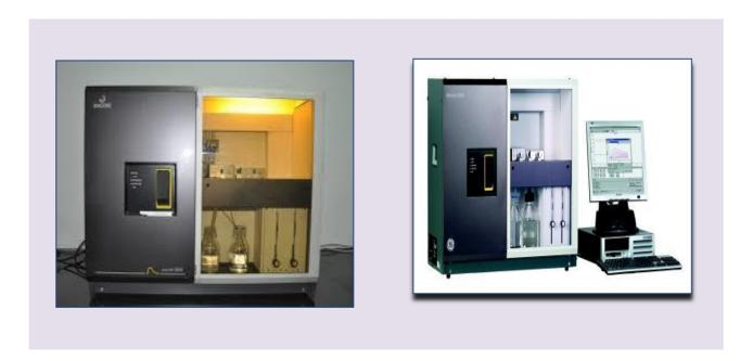
They are two very robust SPR instruments. These instruments use a single chip with four surfaces to which different molecules can be attached, making it possible to simultaneously determine 3 different affinities.
