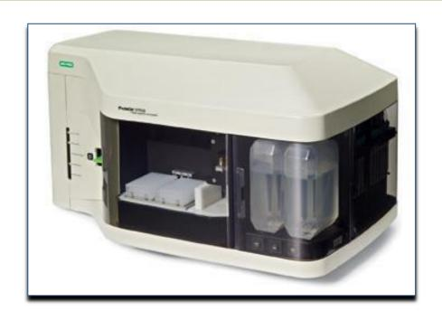
ProteonXPR36 is array based system with funds from the DBT-IISc partnership program. This allows for one shot kinetics and can have upto 36 ligands immobilized on the chip surface and has greatly increased the throughput of the facility.
