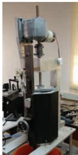
The Couette Cell and apparatus to conduct experiments to understand vortex flow in sheared granular materials (Krishnaraj KP and **Nott PR**. A Dilation-Driven Vortex Flow in Sheared Granular Materials Explains a Rheometric Anomaly. *Nature Communications*. 2016. 7:10630).
