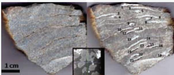
Spheroidal weathering of a diabase in hand-specimen scale. (Banerjee A, **Chakrabarti R** and Mandal S. Geochemical Anatomy of a Spheroidally Weathered Diabase. *Chemical Geology*. 2016. 440:124-138).
