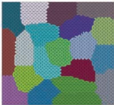
When a system becomes more complex, predicting its behaviour becomes computationally daunting. This problem has now been addressed by decomposing the physical domain, thus increasing the computation speed (Pranesh S and **Ghosh D**. Addressing the Curse of Dimensionality in SSFEM Using the Dependence of Eigenvalues in KL Expansion on Domain Size. *Computational Methods in Applied Mechanics and Engineering*. 2016. 311:457-475).
