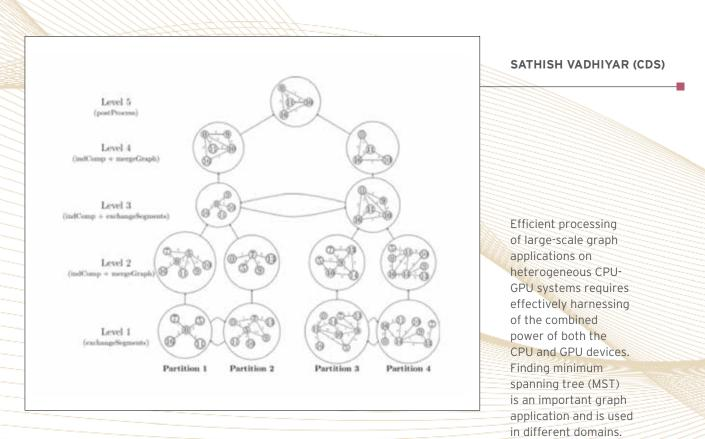
In this research, a multi-node multi-device algorithm is proposed for MST, MND-MST). algorithm exhibits almost linear scalability for large size graphs and shows that the use of GPUs result in up to 23% improvement in performance over multi-node CPU-only performance.
