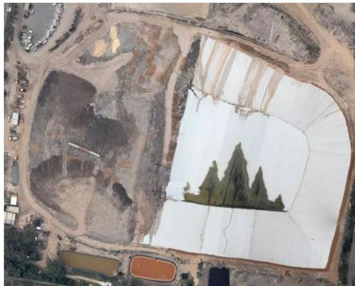
**Figure 8:** Plain view of Landfill cell before placement of drainage layer; Note: Photo was taken on 20/02/2010.
