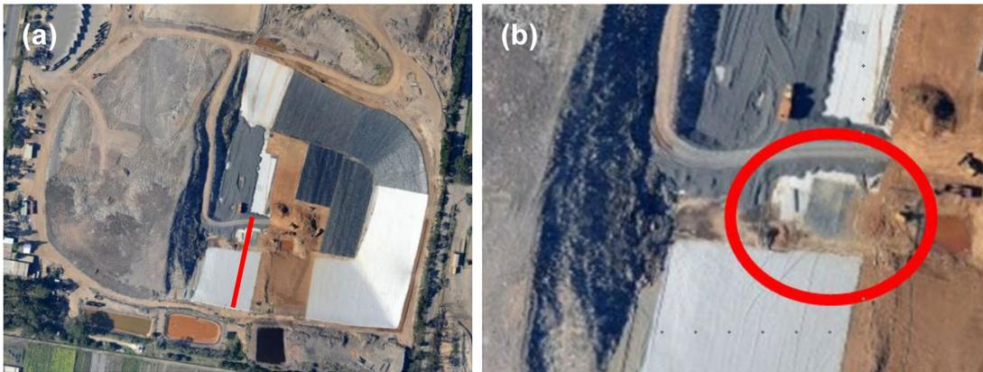
**Figure 7:** Plain view of landfill cell during construction. Note: **a** the red line shows the indicative location of the temperature probes; **b** geomembrane exposed inside the red circle. Photo was taken on 07/01/2010.
