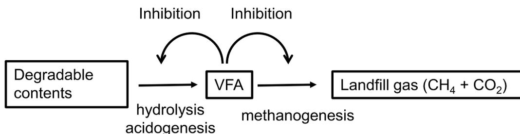
**Figure 1:** Two-stage anaerobic degradation model.
