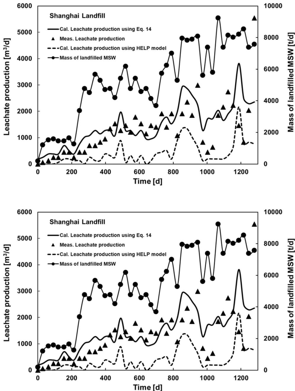
**Figure 9:** Comparison of different leachate production calculation models and the measured values.
