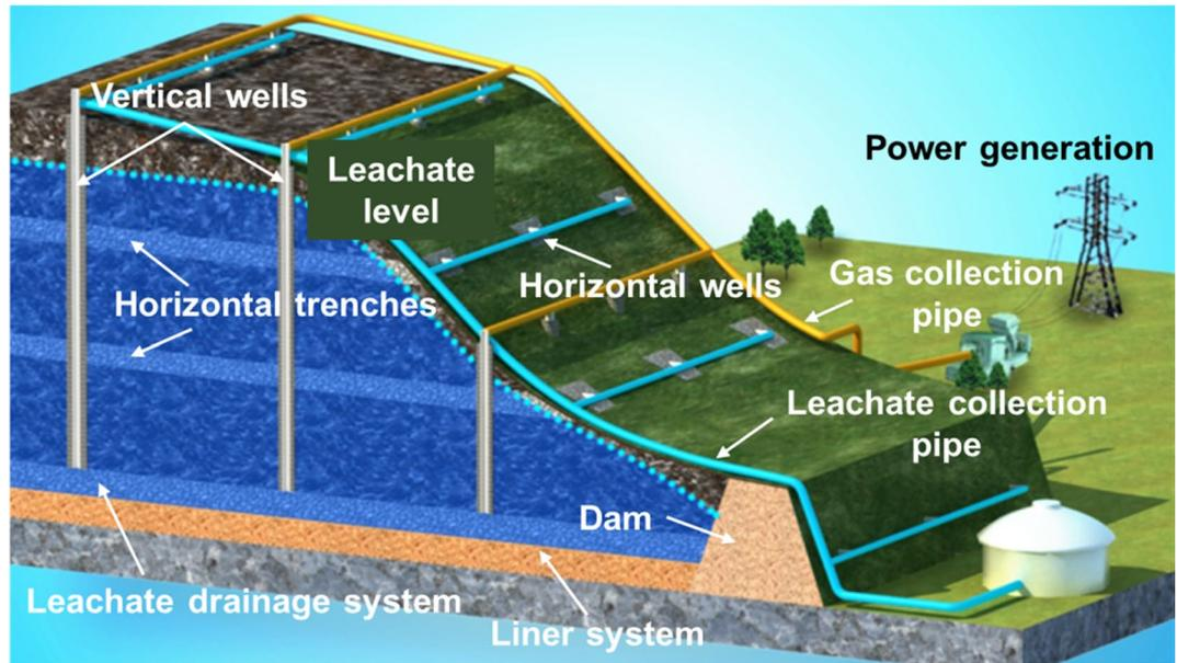
**Figure 10:** Concept of the 3-dimensional drainage system of a landfill with a high leachate level.
