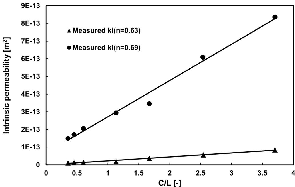
Figure 8: Intrinsic permeability variation with degradation:  $k_i$  vs.  $C/L$ .
