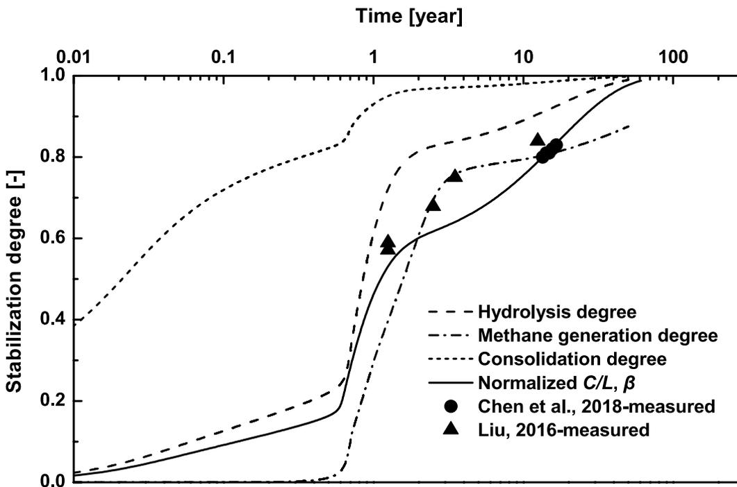
Figure 3: The stabilization degree of HFWC MSW and comparison of calculated and measured  $\beta$  values<sup>11</sup>.
