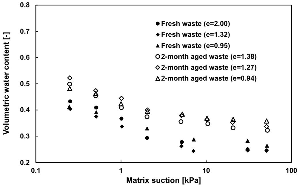
Figure 7: The soil–water characteristic curves of fresh and 2-month aged MSW.
