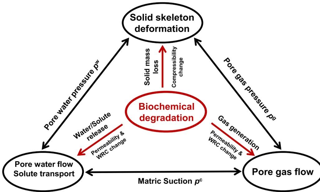
Figure 2: Degradation-consolidation model of landfilled MSW<sup>11</sup>.
