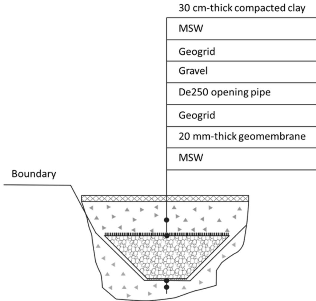
**Figure 12:** Structural diagram of the horizontal trench.
