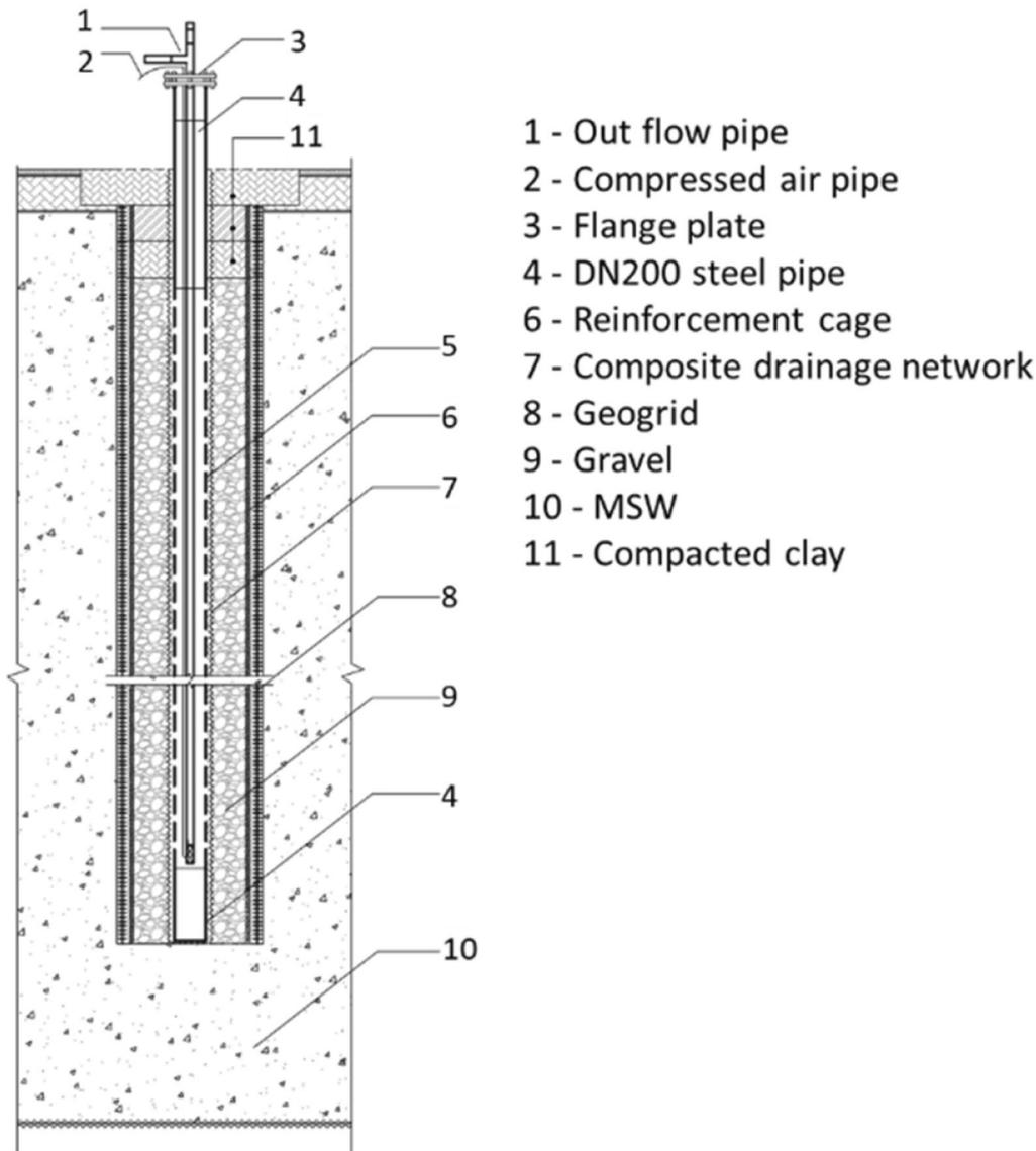
**Figure 11:** Structural diagram of a large-diameter vertical well.
