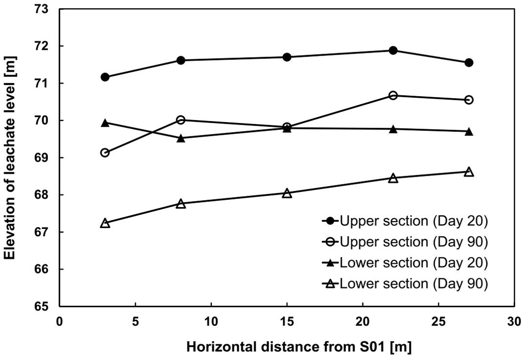
Figure 14: Pore pressure changes after drainage using horizontal well.
