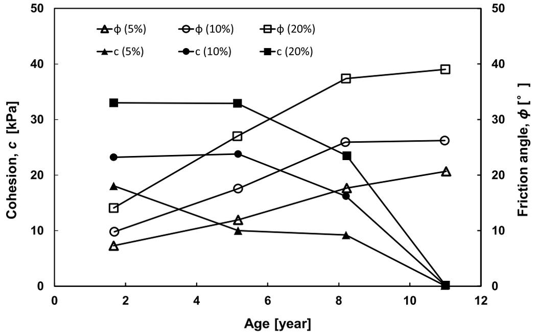
Figure 5: The influence of degradation on the strength properties of MSW<sup>17</sup>.
