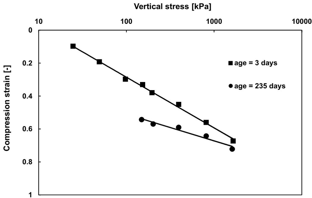
**Figure 4:** Compression curves of fresh and degraded MSW.
