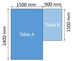
2. Dimensions of tabletop: (A) 2400\*1500\*300 mm (8feet\*5feet\*12inches) + (B) 1500\*900\*300 (5feet\*3feet\*12inches), thickness in the range 300-320mm.
