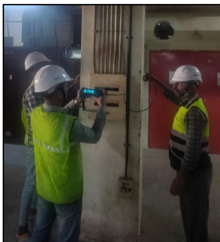
Ultrasonic Pulse Velocity test on RC column and beam in progress
