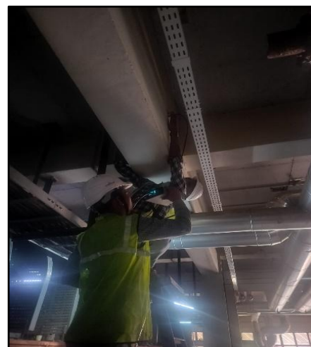
Ultrasonic Pulse Velocity test on RC column and beam in progress
