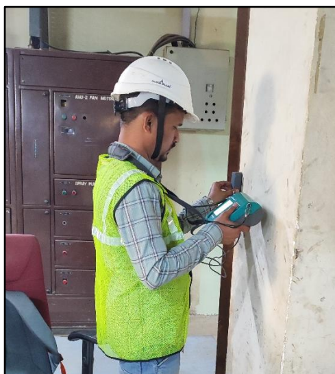
Cover meter studies on RC columns in progress
