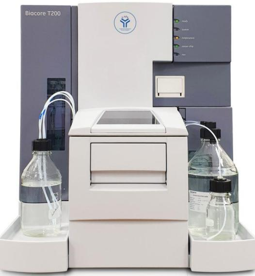
They are two very robust SPR instruments. These instruments use a single chip with four surfaces to which different molecules can be attached, making it possible to simultaneously determine 3 different affinities.
