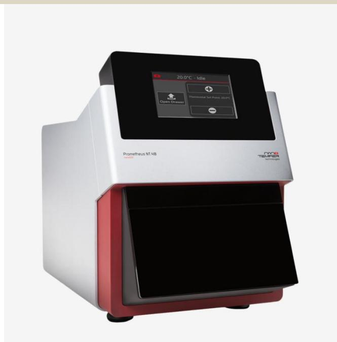
Prometheus NT.48 is a protein stability analysis instrument from NanoTemper Technologies that uses nanoDSF (nano Differential Scanning Fluorimetry) to measure thermal and chemical stability of proteins in a label-free way. It monitors intrinsic tryptophan and tyrosine fluorescence as proteins unfold when heated or exposed to
