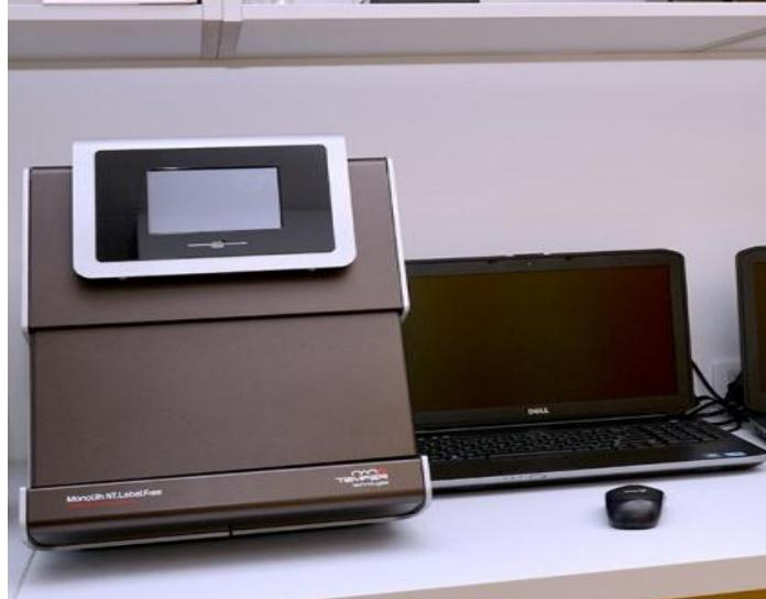
Monolith NT.115 is a laboratory instrument from NanoTemper Technologies that uses MicroScale Thermophoresis (MST) to precisely measure biomolecular interactions and binding affinities in solution. MST works by creating a tiny temperature gradient with an
